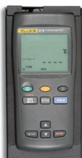
FLUKE METER 51 II CANNOT DOWNLOAD TO COMPUTER
