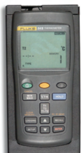
FLUKE METER 53 II COMPUTER DATA LOGGING, CAN DOWNLOAD TO COMPUTER
